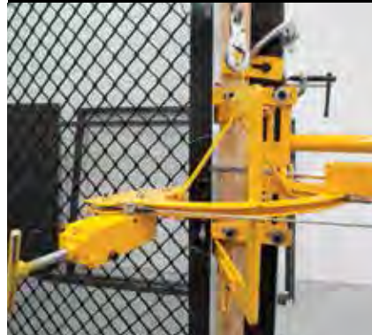
This internal test simulates an attack with a screwdriver.
